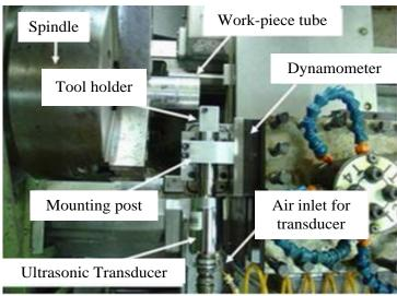
Fig.3 Ultrasonic vibration machining devices<sup>[15]</sup>
