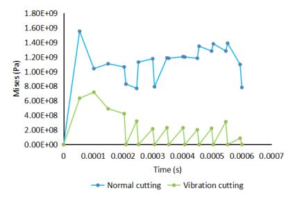
Fig.6. The stress of normal cutting and vibration cutting
