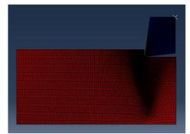
Fig.2 Contact between the workpiece and tool in ultrasonic vibration cutting model
