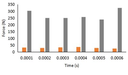
Vibration cutting Normal cutting Fig.5. Cutting force
